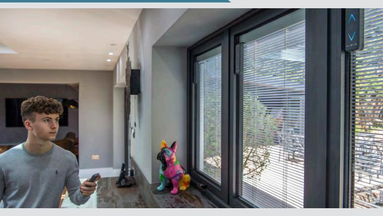
Wire-free solar powered, eco-friendly simplicity is at the heart of the advanced W Smart system with ScreenLine® inside. This system enables a Venetian blind encapsulated within a double-glazed unit to be raised, lowered and slat tilted via a single control device attached to the window, or by remote control. Suitable for both residential and commercial environments, W Smart is sleek, maintenance-free and available for Uni-Blinds® integral blinds within 20, 22, 27 or 29mm cavities.
